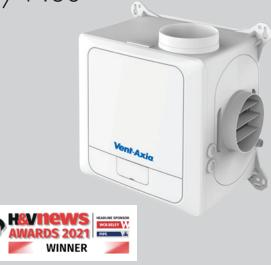
Sentinel Multivent continuous mechanical extract ventilation, MEV is designed for the simultaneous ventilation of separate areas in the home or as a multipoint extraction system for a wide range of commercial applications. The units can be wall, ceiling or loft mounted. Where the ambient air has a high humidity content condensate drains are provided.
